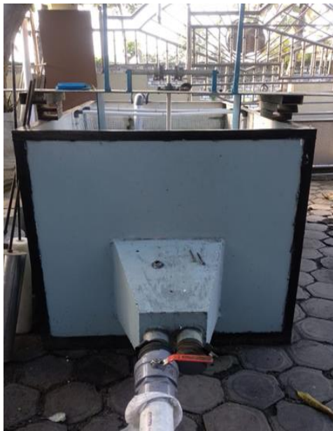
Gambar 8. Flow Tank Tampak Depan
