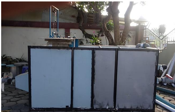
Gambar 7. Flow Tank Tampak Samping
