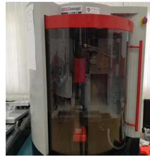
Gambar 4. Mesin CNC EMCO Mill 55 [22]
