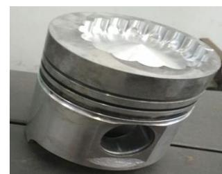
Gambar 4. LSCS piston chamber
