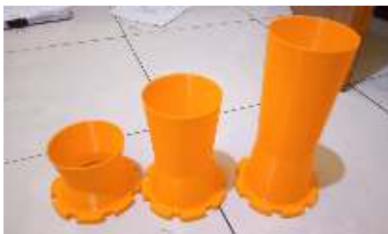
Gambar 8. Hasil Manufaktur Outlet Duct CD 75mm, 150mm, 225mm
