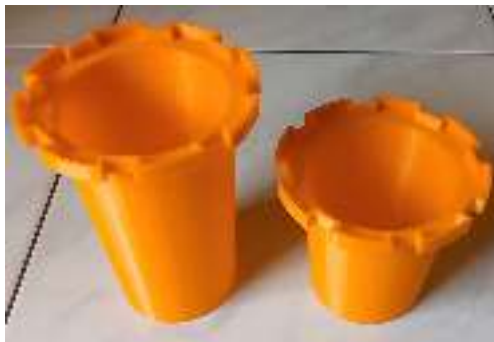
Gambar 7. Hasil Manufaktur Outlet Duct Convergent 100mm dan 150mm
