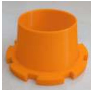
Gambar 6. Hasil Manufaktur Outlet Duct Convergent 50mm
